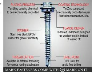
As per the standards MARK fasteners are considered to be a better option for building in environment exposed to corrosive elements.
